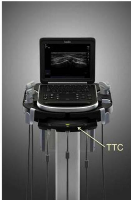
**Fig. 13.** Triple transducer connector (TTC) on a SonoSite bedside ultrasound machine. (Courtesy of FUJIFILM Sonosite Inc; with permission.)
