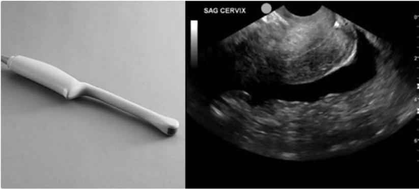
Fig. 17. Intracavitary probe and corresponding ultrasound image.
