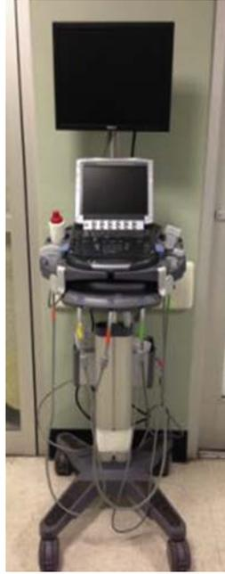
**Fig. 8.** Ultrasound machine with teaching or secondary viewing screen mounted on the portable stand.
