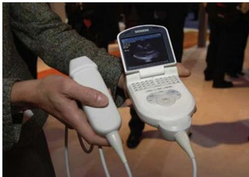
**Fig. 1.** Portable handheld ultrasound machine Acuson P-10. (Courtesy of Siemens Healthcare Copyright 2013; with permission.)
